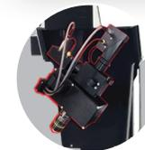
**FEMTO SMART** microscopes equipped with a motorized tilting module provide a higher level of freedom to reach the sample from different angles by rotating the objective.
